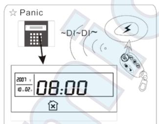
Press the panic button on remoter, or press "confirm/panic" key on panel for 3 seconds, and 10 seconds later the panel will dial the preset phone number. And you can disarm to cancel alarm.
